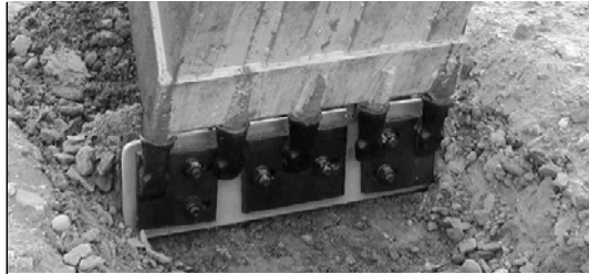
Bolt on Finishing Edge System
