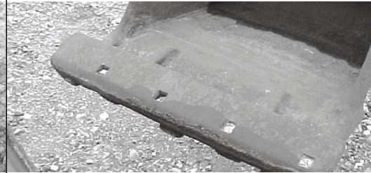
traditional weld-on finishing edge
